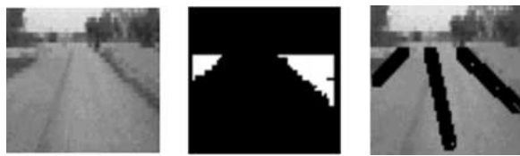
Figure 29. Segmentation and edges estimation on cloudy conditions.
