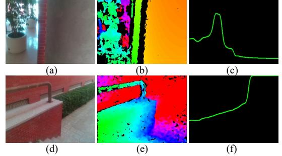
Figure 4. (a)(d) Color images; (b)(e) Depth maps; (c)(f) Traversable lines.
