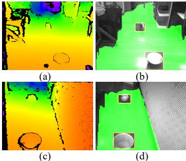
Figure 5. Low-lying obstacle detection and traversable area segmentation: (a)(c) Depth maps in fake color; (b)(d) Low-lying obstacle detection results by producing bounding windows and traversable area segmentation results by producing the green mask to overlay on the IR images.
