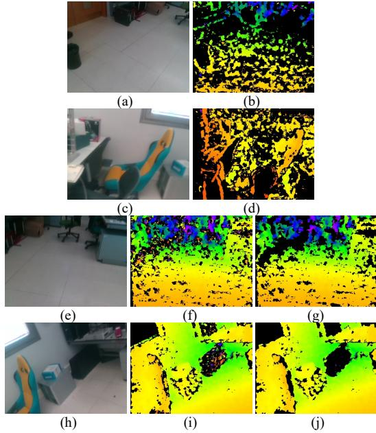
Figure 3. Color images and depth maps from the wearable smart glasses: (a)(c)(e)(h)Color images; (b)(d) Original depth maps; (f)(i) Depth maps with dense preset configuration; (g)(j) Denoised depth maps.
