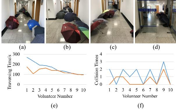
Figure 7. Field test: (a-d) test scenario; (e)f) experiment data sorted in descending orders of the traversing time while the blue lines are collected with traversability awareness and the orange lines are collected with traversability awareness and low-lying obstacle detection.
