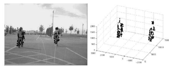
Fig. 1. (Left) Two-dimensional points overlayed on left image. (Right) Three-dimensional coordinates of detected pixels.
