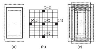
Fig. 2. MC generation approach. (a) Oversized and downsized windows. (b) Spatial centers for each window. (c) Fifteen candidates are generated.
