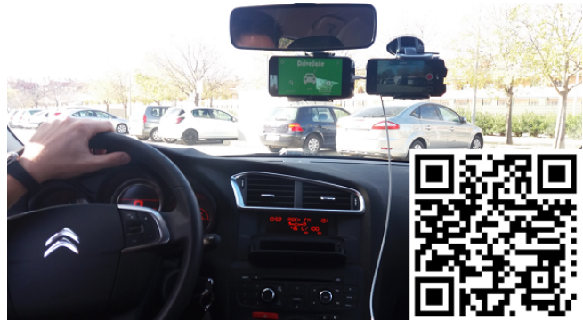
Fig. 1. DriveSafe and video-recorder on one of the testers windshield.
