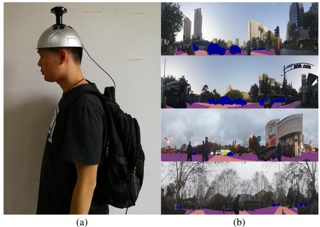
Fig. 4. (a) Wearable navigation assistance system; (b) Unfolded panoramas with annotations.
