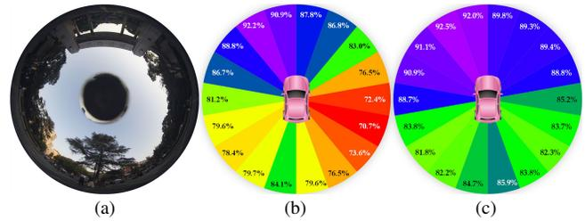
Fig. 6. (a) A raw panoramic annular example image to indicate the orientation, (b) Segmentation accuracy values in different directions without data augmentation, and (c) with all data augmentations.
