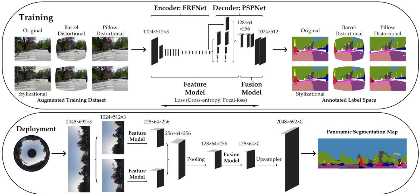
Fig. 2. The proposed panoramic annular semantic segmentation framework.
