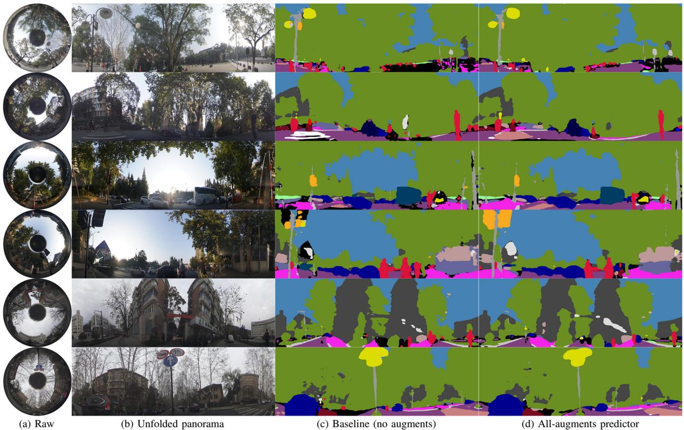
Fig. 7. Qualitative examples of panoramic annular semantic segmentation: (a) Raw panoramic annular images, (b) Unfolded panoramic images, (c) Segmentation maps without data augmentation, and (d) with data augmentation.
