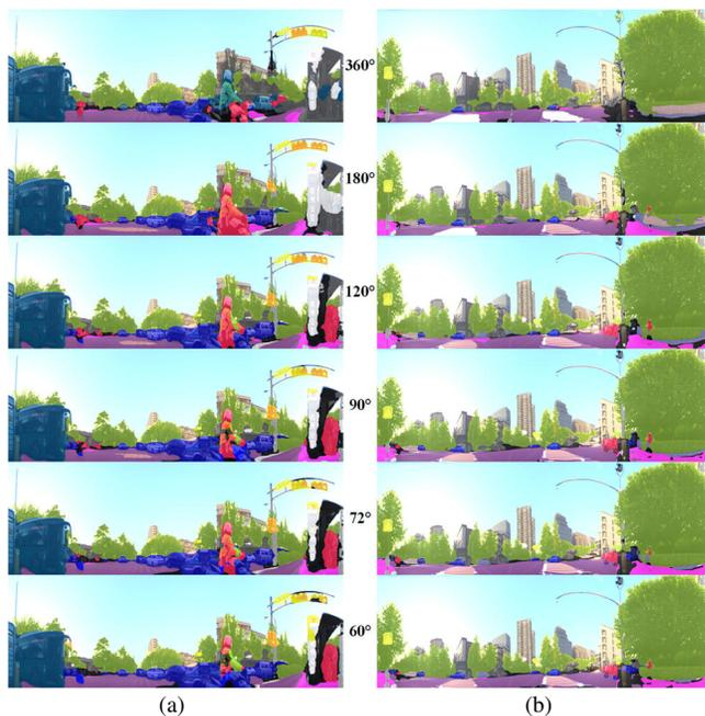
Fig. 5. Qualitative examples of semantically masked panoramic images by using our augmented PASS framework with different inference settings. From top to bottom: 360°-per-segment, 180°-per-segment, 120°-per-segment, 90°-per-segment, 72°-per-segment and 60°-per-segment results.
