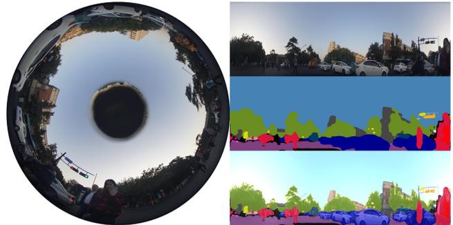
Fig. 1. The proposed panoramic semantic segmentation on real-world surround image captured by our panoramic annular lens system.
