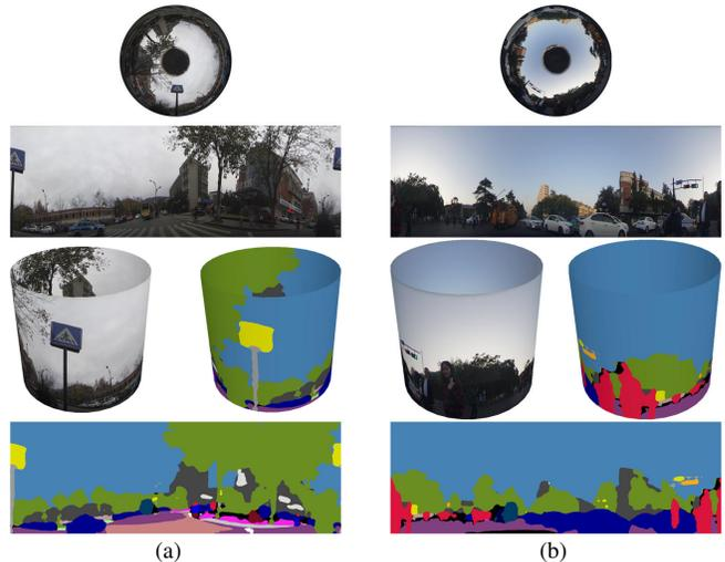
Fig. 3. Panoramic annular images can be folded back into  $360^\circ$  cylindrical rings for seamless padding and upsampling.
