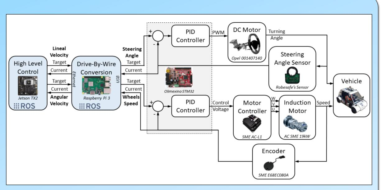
Next, the Throttle-By-Wire system was implemented. Being an electric car this stage was easier. The acceleration of the car is controlled by a continuous voltage that is sent to the AC Induction Motor Controller of the propulsion engine of the car. This control voltage is generated through the development board. An encoder was installed in the propulsion engine to feed back the motor speed.
