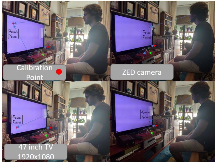
Fig. 2: Calibration step. The user under test has to watch during 8 seconds 4 points displayed on the screen
