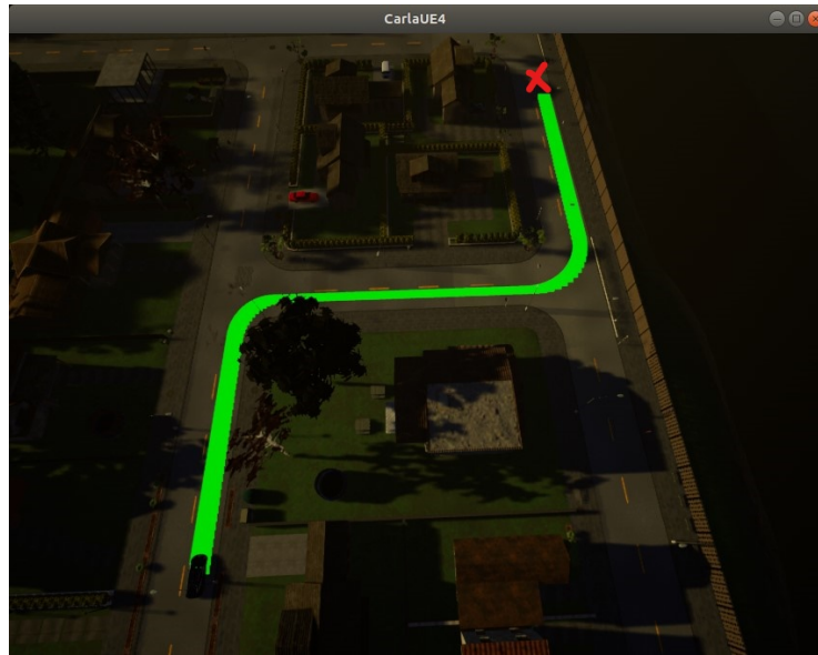
Fig. 10. Navigation-trajectory on CARLA's Town01 scene obtained by Global Path Planning A* algorithm provided by Carla PythonAPI.
