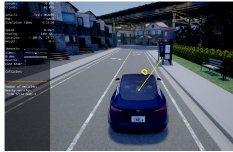
Fig. 5. Unexpected Pedestrian scenario. The pedestrian can be found behind the bus stop, so the perception systems detects it at the moment it is entering the road
