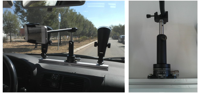
(a) System mounted on the vehicle. (b) Electromechanical goniometer.
