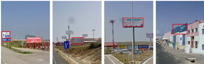
Fig. 8. Panel detection under cluttered background. The two leftmost images are correct detections and the rightmost images are false positives.
