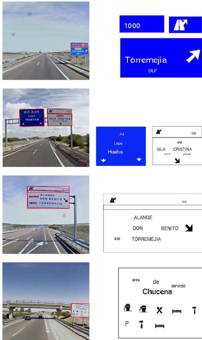
Fig. 11. Image results. Panel detections are on the left column and text recognition on the right column.
