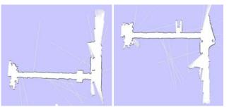
Fig. 4. Partial maps built by robots.
