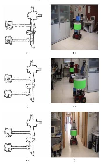
Fig .7. Collaborative multi-robot Monte Carlo localization.
