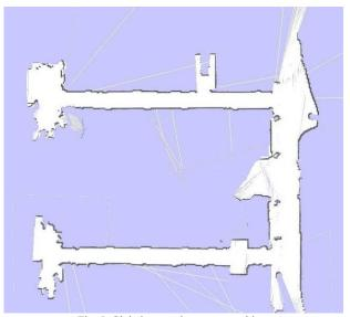
Fig. 5. Global map using scan-matching.
