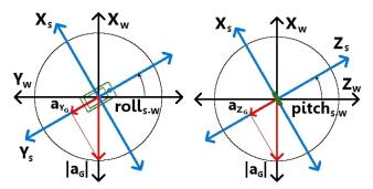
(a) Gravity acceleration on  $Y_S$ . (b) Gravity acceleration on  $Z_S$ .
