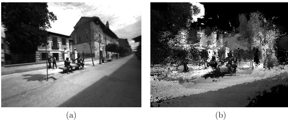
Figure 2.14: Example of a dense 3D reconstruction in the city of Alcalá de Henares. (a) Image view of the Cervantes house area (b) Reconstructed dense 3D point cloud.
