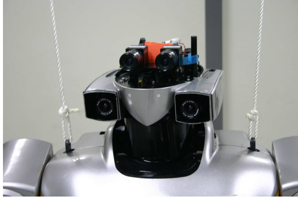
Figure 5.3: HRP-2 stereo rig settings. In this work we consider the two cameras attached to the ears that have a baseline of approximately 14.4 cm.
