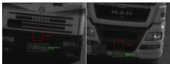
Fig. 12. Some examples of vehicle logo recognition errors in trucks due to the high distance between the license plate and the logo.
