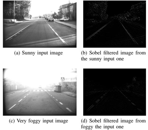
Figure 2: Sobel images in different fog states
