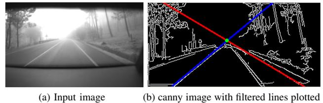
Figure 3: Canny-filtering, Hough line detection with filtered parameters and vanishing point calculation
