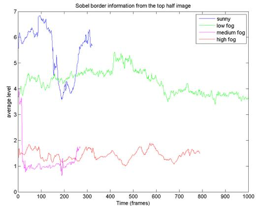
Figure 6: Sobel statistics in various levels of fog
