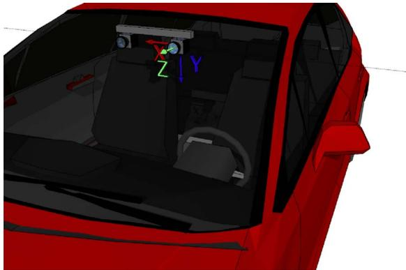
Fig. 1. Camera coordinate system.
